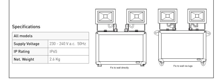
The Twin LED Spotlight can be fixed to the wall either directly or using the lugs provided.
